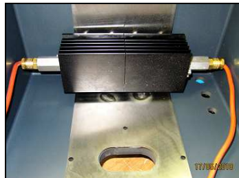
Enclosure Exd Heater 2x type SHR with ALU body
