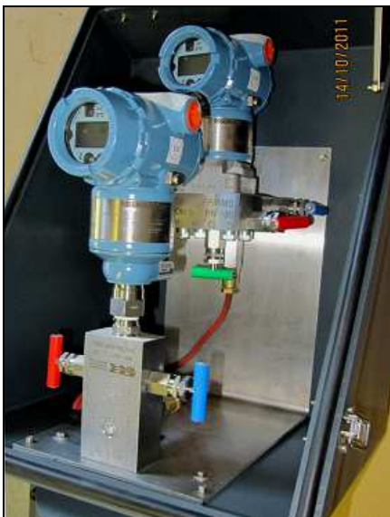
ENCLOSURE S3-1 with window For pressure and differential pressure Transmitter Mounting: Pressure on the bottom with 2-way manifold DP on the wall with 5-way manifold Manifolds are directly heated by Exd SH
