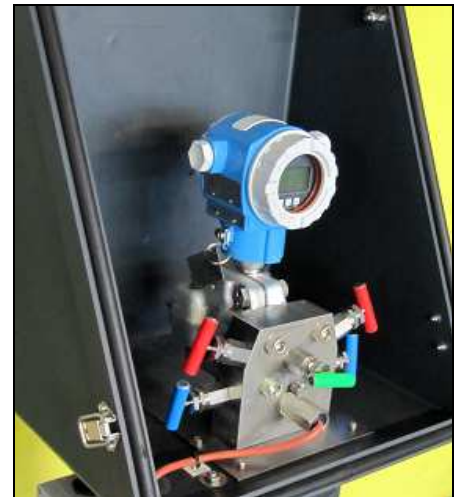
ENCLOSURE S3-1 with window for differential pressure transmitter Mounting on the bottom incl.5 way manifold type SB5SFP directly heated by Exd heater SH
