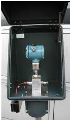
ENCLOSURE S3-1 For pressure transmitter Mounting on bottom Incl. 2 way manifold „SB“ Directly heated by Exd heater SH For transmitter adaptor BFA ½“NPT
