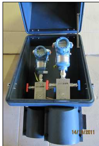
ENCLOSURE S3-1 with window for 2x pressure transmitters Mounting on the bottom 2x 2 way manifold SB2 directly heated by Exd SH
